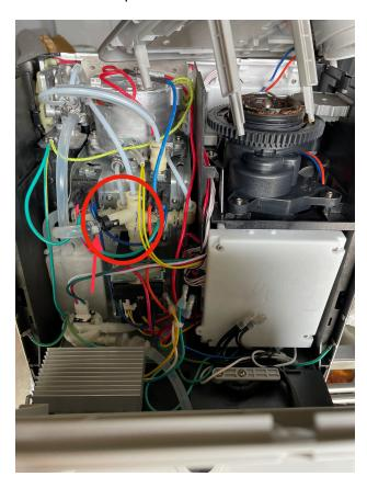
The tube will need to be removed, so cable tie may need to be cut and replaced with a new one. Others said they were able to just stick something small enough to stretch the tie enough to pull tube off, but that will be up to you. I already had cable ties, so I just carefully cut the cable tie off. Be careful to not cut the tube. Once cable tie is removed, you can now remove tubing from valve and separate the clamp. Shown here:
